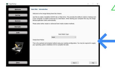
Choose the **Boot Media Type**. Simple is recommended for most users. Advanced is for server operating systems that need to specify RAID controller drivers. Drivers can be loaded after booting PC to the image boot media.
