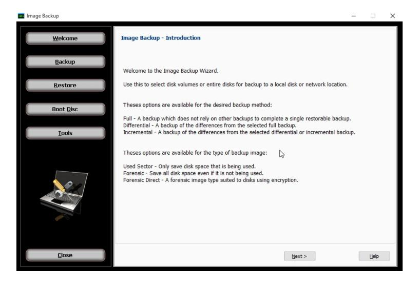
Use the buttons on the left side of the screen to manually perform an image backup or restore operation, create a boot disc, or access various disk image management tools. Creating backup images manually allows more control over where the images are stored and how they are named than do scheduled backup jobs, but requires the user to assume additional responsibility for managing the images.
